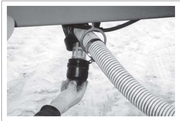
Fig. 41 SCREEN CANISTER (TYPICAL)
