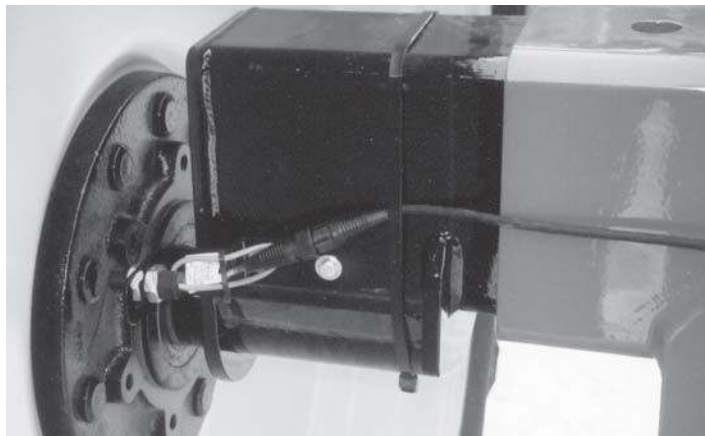
Fig. 21 FIELD Speed Sensor (Automatic System)
