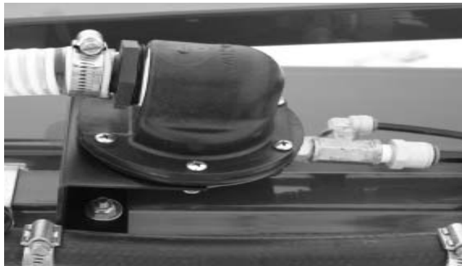
Mixing Chamber is mounted on flip wing
