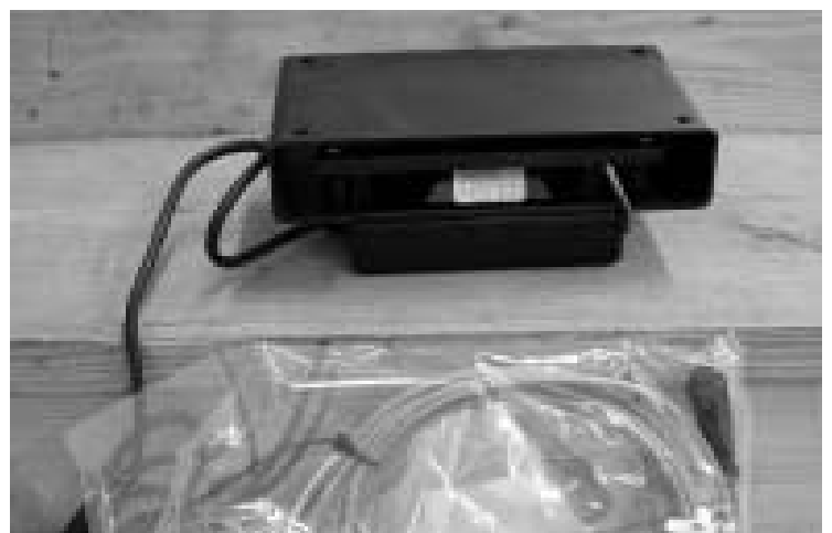
Fig. 46 GROUND SPEED SENSOR RAVEN RADAR
