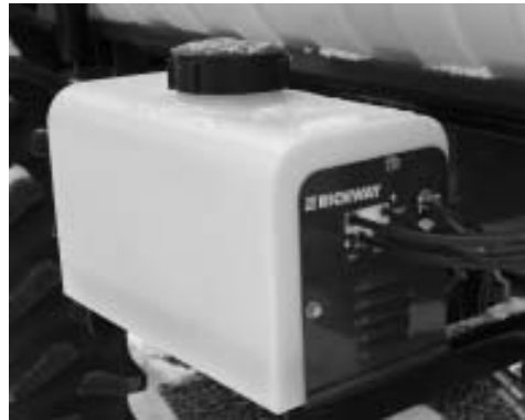
Direct Injection (Foam Concentrate Tank Shown)
