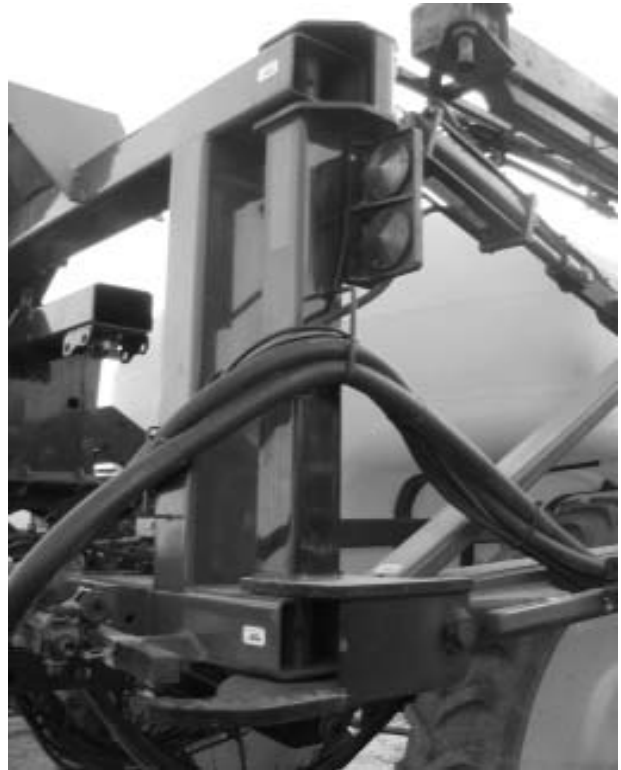
Wing Pivot for 9500 Series 120-132' wings (RH Shown)
