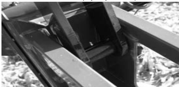
9500 Series 120-132' Flip Wing Linkage (1 zerk per side)
