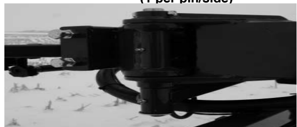
9500 Series 120-132' Swing Wing Pin (2 zerk per pin/side)
