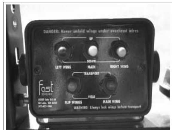
Fig. 14 BOOM POSITION SWITCH BOX 9500 Series 60-100' shown
