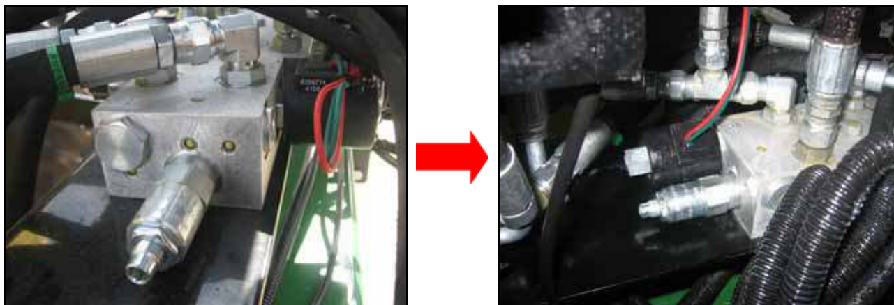
FIGURE 1. Converted Hydraulic Valve - Closed Center to Open Center
