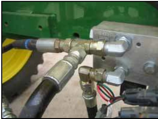
FIGURE 4. Pressure and Tank Hoses Installed
