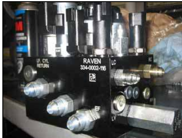
FIGURE 8. Fittings Installed on the AutoBoom Valve
