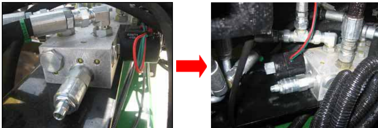
FIGURE 1. Converted Hydraulic Valve - Closed Center to Open Center
