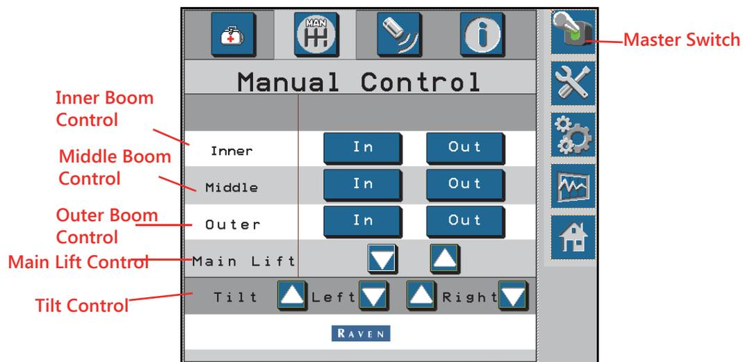
2. Turn the master switch
