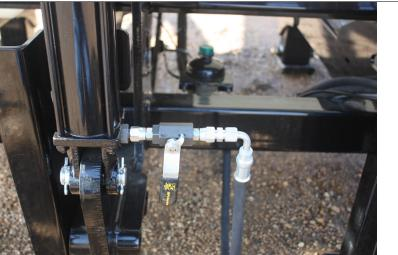
Fig. 55 BOOM CYLINDER VALVE
