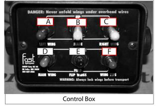
F. Breakaway Wing Switch 80-88-90-100 ft. This spring-loaded-to-neutral-center toggle switch controls the breakaway wing, field to transport function. Move the switch up and hold to fold in the breakaway wing for transport and down to fold out to field position.
