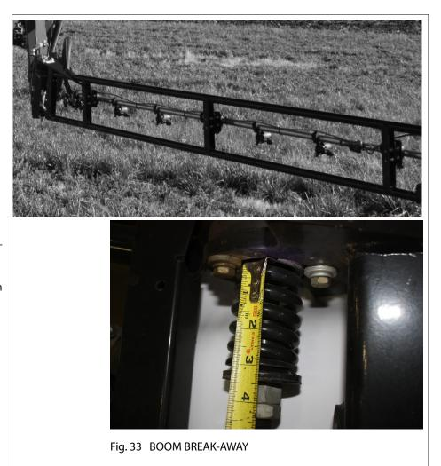
16. Boom Break-Away: Each boom is designed with a breakaway hinge between the outer booms and the boom extention. Each of these hinges will break-away frontwards or backwards when the boom strikes an obstruction to prevent damaging the boom.
