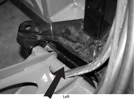
Fig. 62 BOOM TILT PIVOT
