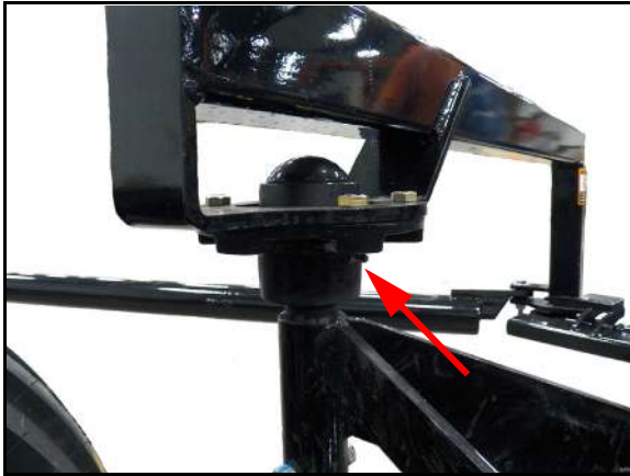
Grease pivot joints annually.
