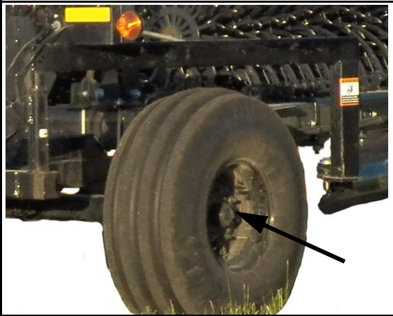
Grease main wheel bearing annually.
