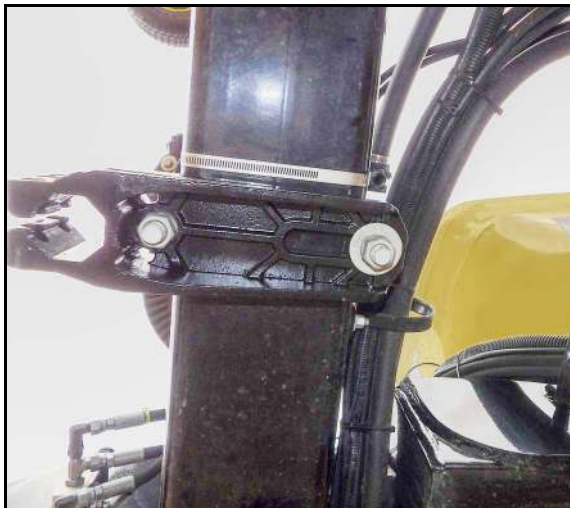
Nut and washer arrangement for Coupler Mount.
