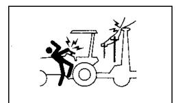
CAUTION: Keep away from overhead power lines. Serious injury or death may result. Proceed cautiously under overhead power lines and around utility poles. Know the transport height of your machine. Electrocution can occur without direct contact with overhead electrical lines.
