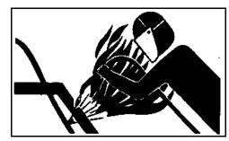
Flammable spray can be generated by heating near pressurized fluid lines, resulting in severe burns to yourself and bystanders. Do not heat by welding, soldering, or using a torch near pressurized fluid lines or other flammable materials. Pressurized lines can accidentally burst when heat goes beyond the immediate flame area.
