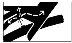
Inspect hydraulic hoses periodically – at least once per year – for leakage, kinking, cuts, cracks, abrasion, blisters, corrosion, exposed wire braid or any other signs of wear or damage.
