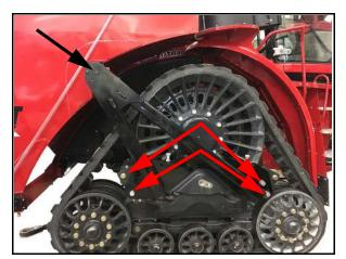
4. Install left side tank mount bracket assembly through the tank receiver to tractor with four 10.9 M24 x 75 mm bolts, lock washers and nuts. Torque to 1000 Nm (740 ft-lbs).
