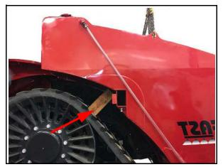
2. Raise tank and guide into tractor as far as possible though the front 3" x 5" cross tube. Lower tank onto axle in rear and brace with a 9.25" long 2x4 between the track and tank.
