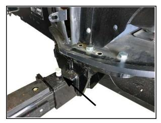
3. Install four 5/8" x 2" bolts and jam nuts into the center tank mount. Tighten the bolts and jam nuts.
