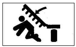
Before operating, make sure air has been bled from wing-fold hydraulic system.
