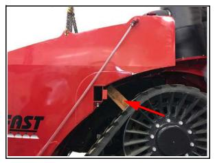
2. Raise tank and guide into tractor as far as possible though the front 3" x 5" cross tube. Lower tank onto axle in rear and brace with a 9.25" long 2x4 between the track and tank.
