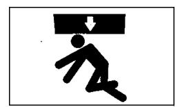
Always use a safety support when working on, under, or around machine. Transport/ Service locks can be used for this purpose.
