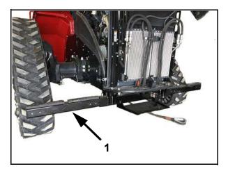
1. Insert front carry tube (1) into receiver tube and center as illustrated.
