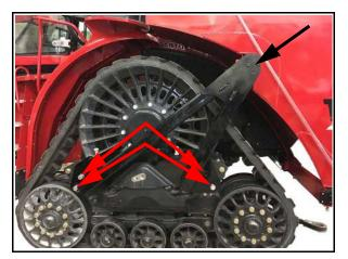
2. Install right side tank mount bracket assembly through the tank receiver to tractor with four 10.9 M24 x 75 mm bolts, lock washers and nuts. Torque to 1000 Nm (740 ft-lbs).
