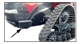
1. Remove toolbox and bracket from the left front of the machine.
