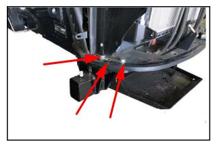
3. Install the hardware with six 10.9 M20 x 90MM bolts, lock washers and nuts and torque to 675 N-m (500 ft-lbs).
