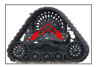
1. Remove the four inner bolts from the track, do not remove the front outer and rear outer bolts.
