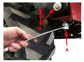
3.Install two 5/8" x 2" bolts and jam nuts (A) into the center tank mount. Tighten the bolts and jam nuts.
