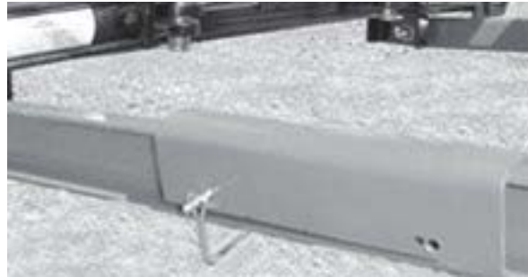
Transport Lock In Storage Position On Boom Stabilizer Arm
