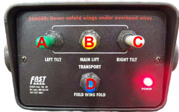
Fig. 1 BOOM CONTROLS (5 FUNCTION BOX) 60 & 66' BOOM
