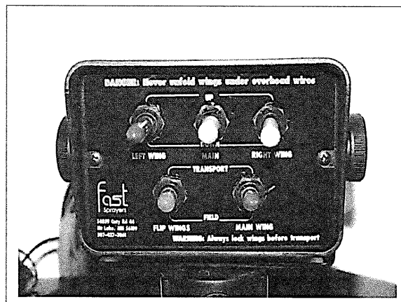
Fig. 14 BOOM POSITION SWITCH BOX
