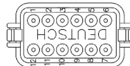
PIN OUT DETAIL FOR PLUG
