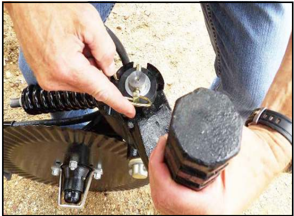
5. Reinstall the washer and pin.
