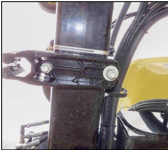
Nut and washer arrangement for Coultter Mount.
