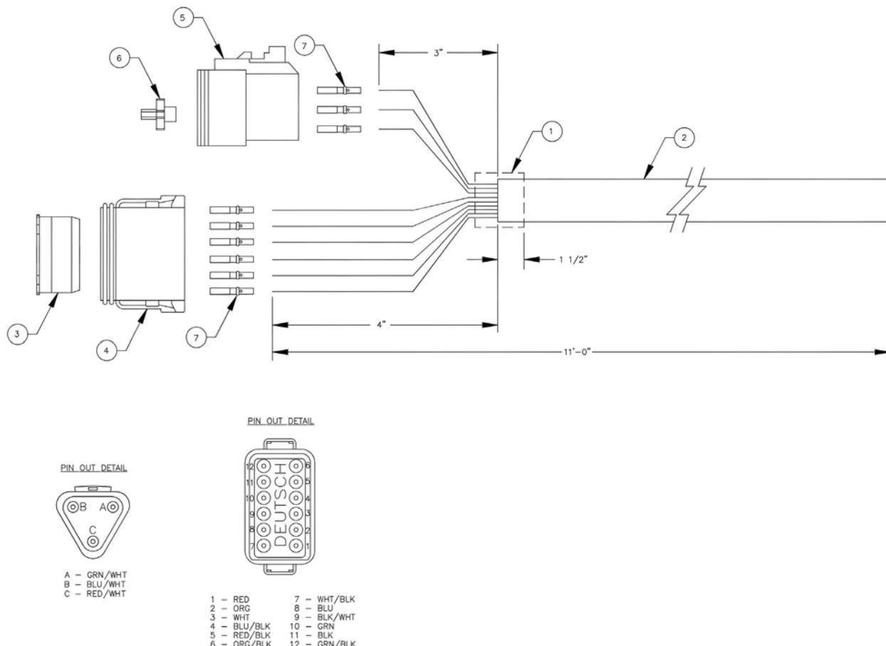
**Wiring Harness - 80, 90 & 100 Foot Boom Parts List**
