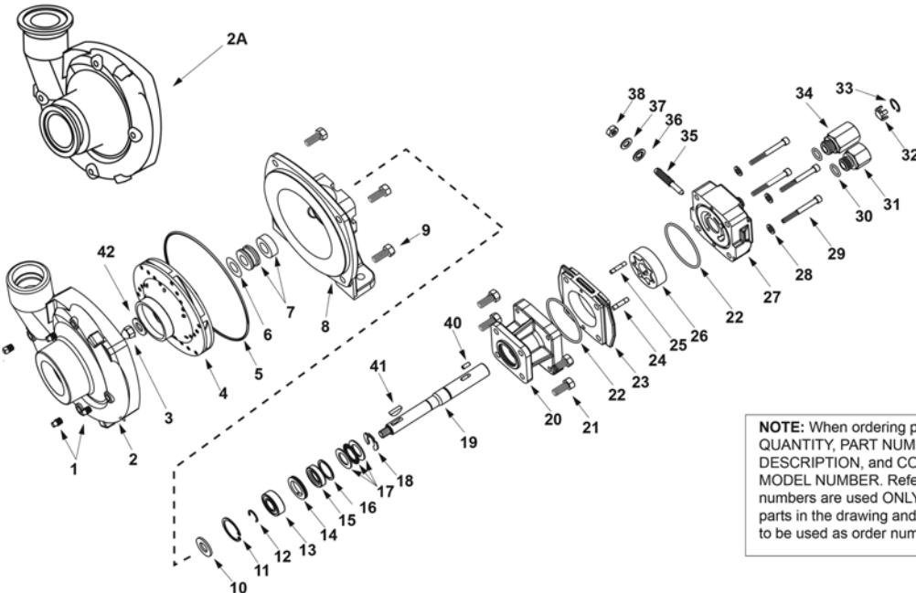
**NOTE:** When ordering parts, give QUANTITY, PART NUMBER, DESCRIPTION, and COMPLETE MODEL NUMBER. Reference numbers are used ONLY to identify parts in the drawing and are NOT to be used as order numbers.
