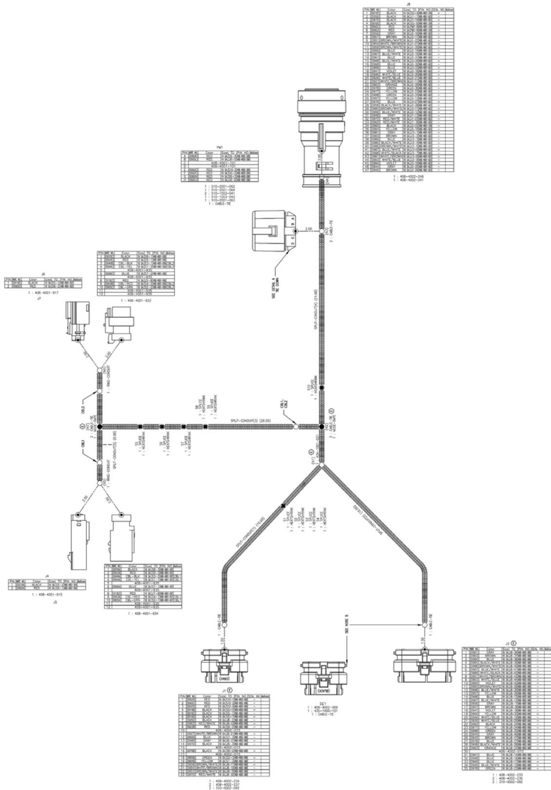
**Cable, 81 Pin ECU, 47 Pin Rate Control Interface (632029)**
