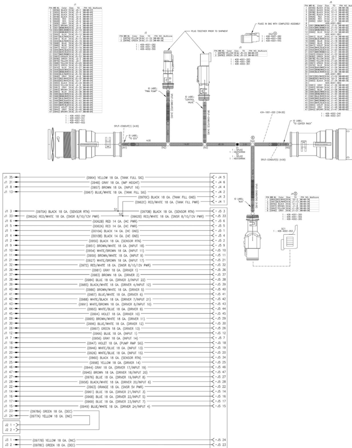
Cable, Pull Type Sprayer Frame, 14' 47 Pin To 47 Pin (632035)
