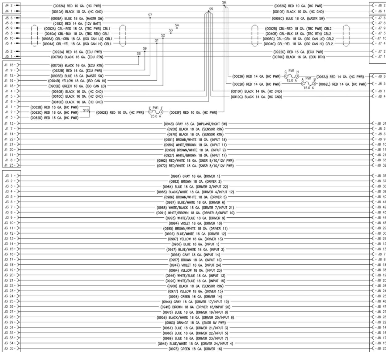
**Cable, Pull Type Sprayer Frame, 14' 47 Pin To 47 Pin (632035)**
