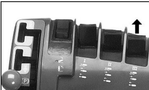
Figure 13: SCV III Pushed Forward
