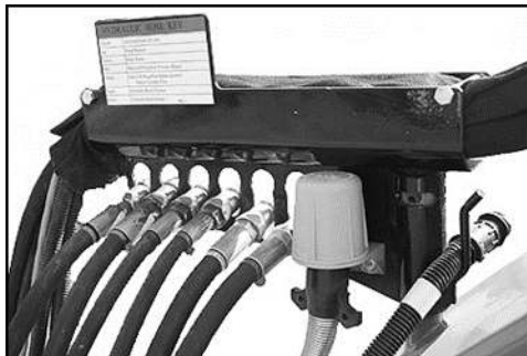
Figure 4: Wiring Harness and Hoses in Storage Position
