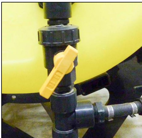
Figure 15: Control valve in normal working position
