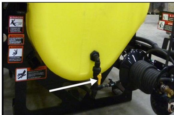
Figure 14: Agitation Pump control valve
