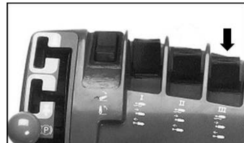
Figure 11: SCV III Pulled Backward
