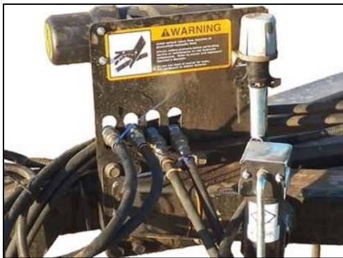
Figure 2: Wiring Harness and Hoses in Storage Position
