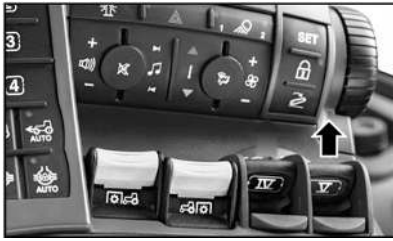
Figure 17: SCV V Pushed Forward
