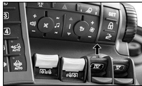
Figure 15: SCV IV Pushed Forward
