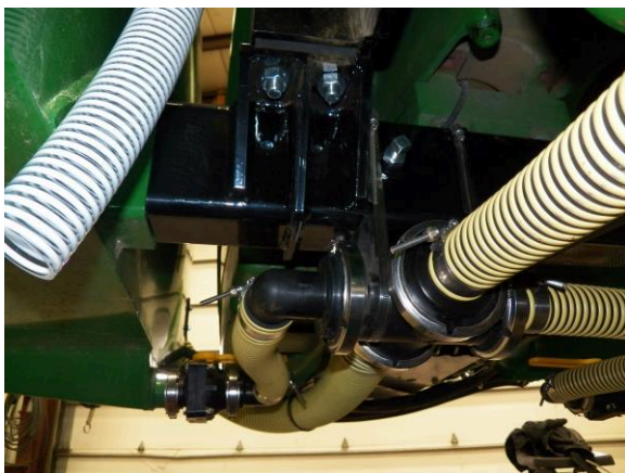
Figure 6: Under-frame plumbing assembly viewed from rear-left.
