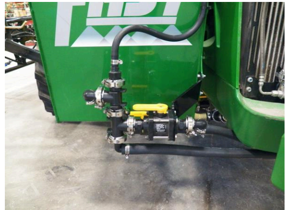
Figure 1: Right-hand tank plumbing assembly
