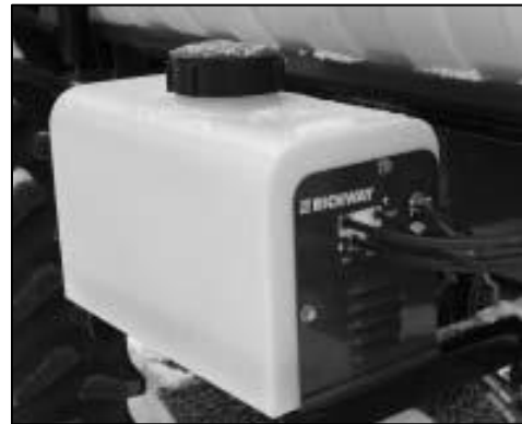
Figure 10: Direct Injection Foam Concentrate Tank
