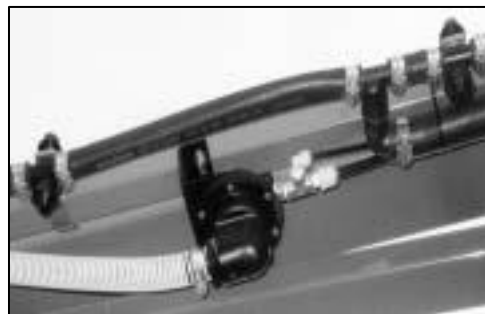
Figure 11: Mixing chamber mounted on the wing
