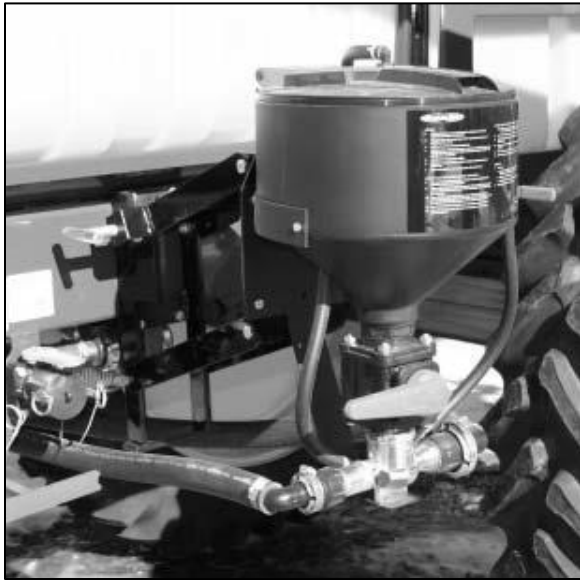
Figure 8: Chemical Eductor in the up position
