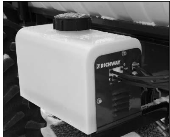
Figure 17: Direct Injection Foam Concentrate Tank
