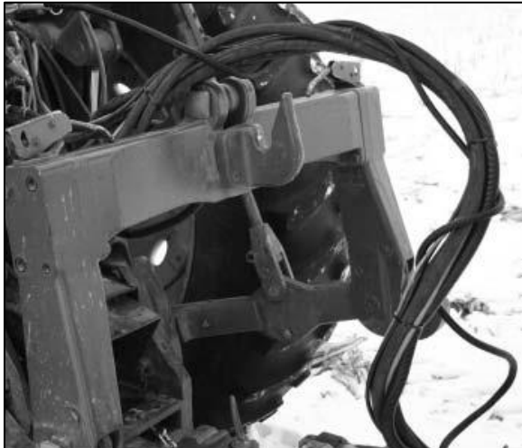
Figure 23: Hydraulic hoses and electrical lines retained
