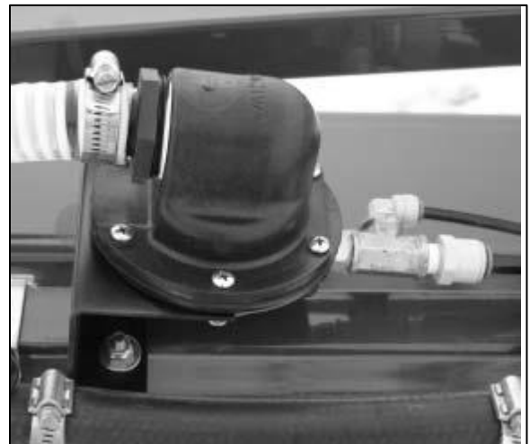
Figure 18: Mixing Chamber is mounted on the flip wing
