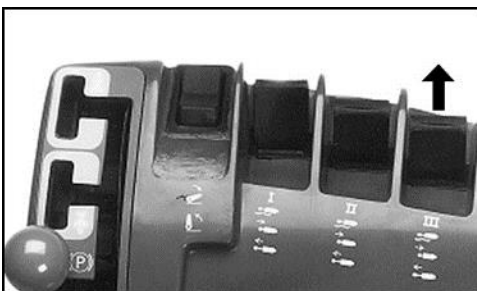
Figure 17: SCV III Pushed Forward
