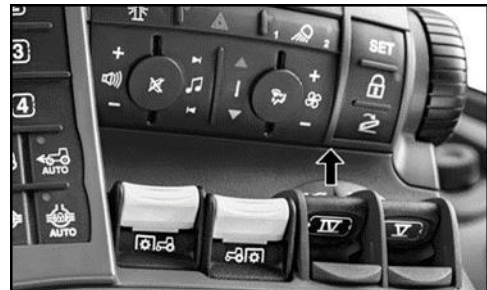
Figure 19: SCV IV Pushed Forward
