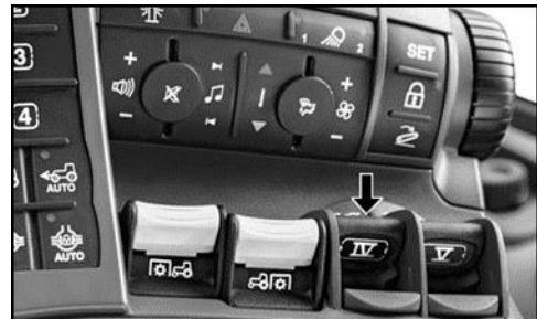
Figure 20: SCV IV Pulled Backward
