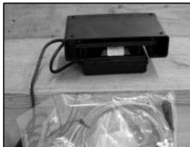
Figure 6: Raven TYP Radar ground speed sensor
