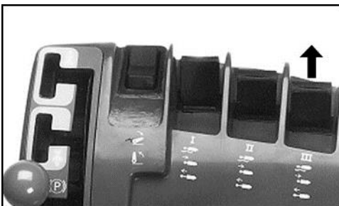
Figure 17: SCV III Pushed Forward
