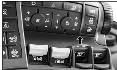
Figure 19: SCV IV Pushed Forward
