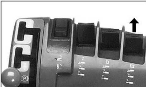
Figure 11: SCV III Pushed Forward
