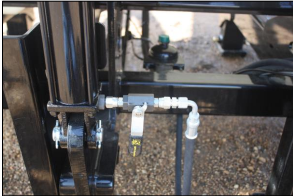
Figure 6: Boom cylinder valve
