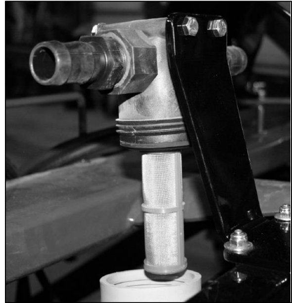
Figure 22: Typical boom line filter/strainer
