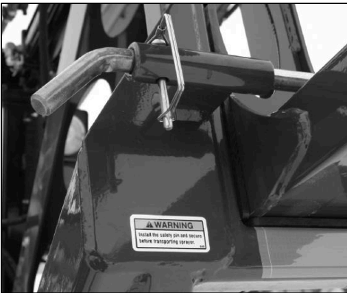
Figure 8: Transport lock pins (both sides)
