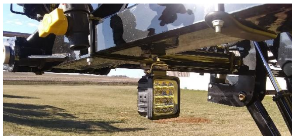
Figure 4: Blue light on rectangular boom
