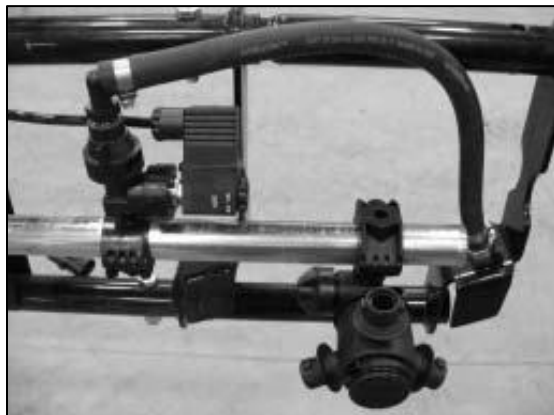
Figure 3: Electric shutoff fence row nozzle
