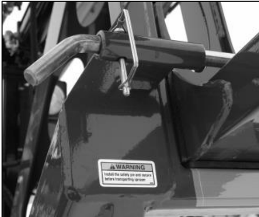
Figure 10: Transport lock pins (both sides)
