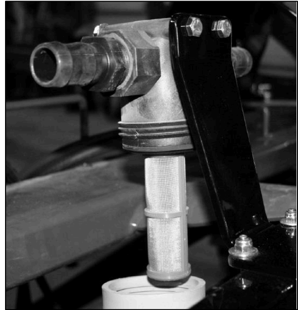
Figure 22: Typical boom line filter/strainer
