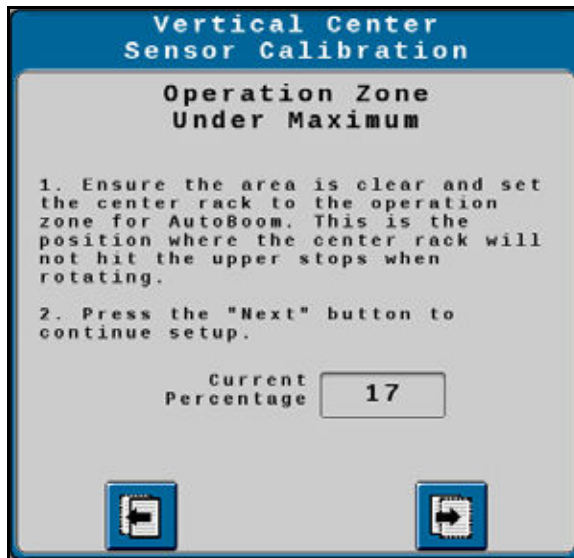
FIGURE 28. Vertical Center Sensor Calibration - Operation Zone
