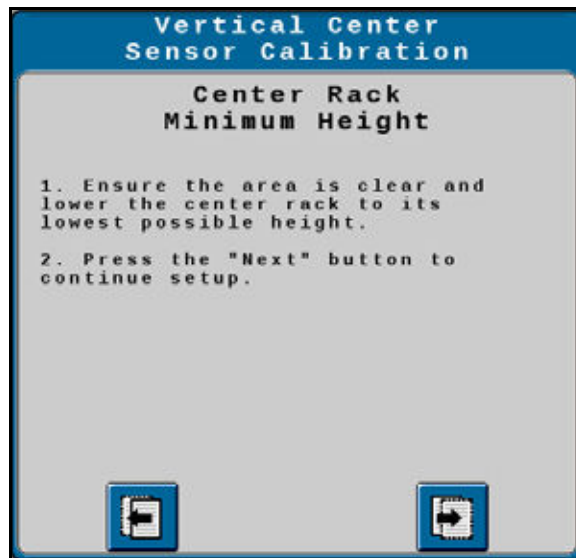
FIGURE 30. Vertical Center Sensor Calibration - Minimum Height
