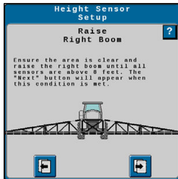
FIGURE 18. Height Sensor Setup - Raise Right Boom
