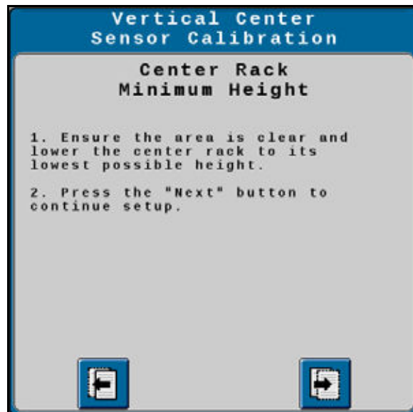
FIGURE 9. Vertical Center Sensor Calibration - Minimum Height
