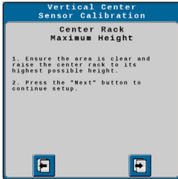
FIGURE 27. Vertical Center Sensor Calibration - Maximum Height
