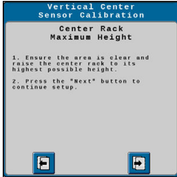
FIGURE 6. Vertical Center Sensor Calibration - Maximum Height
