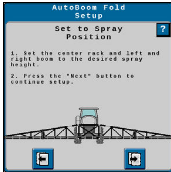
FIGURE 8. Vertical Center Sensor Calibration - Set to Spray Position
