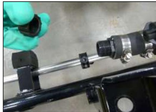
1. Remove the line caps at the end of the stainless-steel wet booms.
