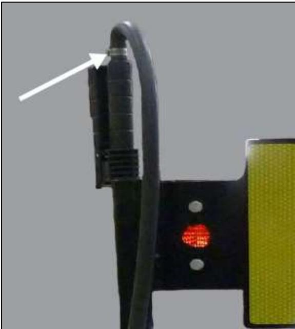
3. Place the end of the hose in a pail to allow fluid to drain.
