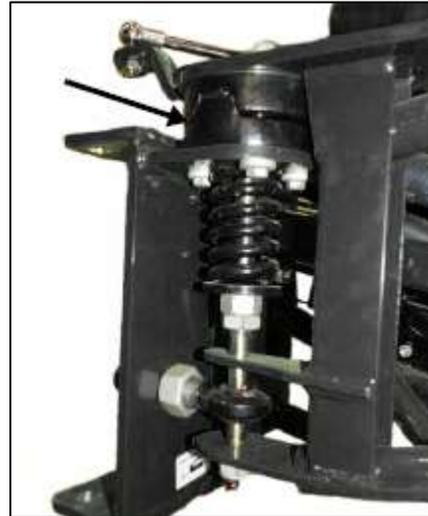
Figure 13: Breakaway clutch
