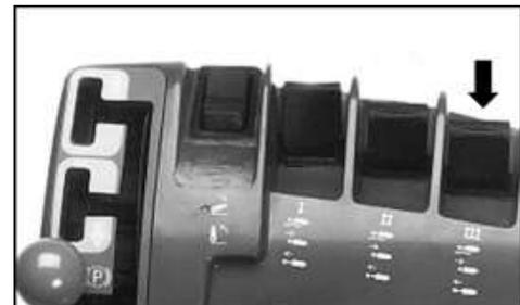
Figure 11: SCV III Pulled Backward
