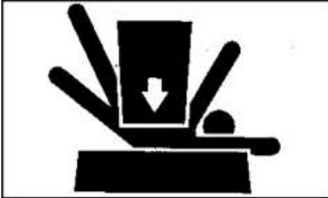
Always lower the attachment or implement to the ground before you work on the machine. If the work requires that the machine or attachment be lifted, provide secure support for them. If left in a raised position, hydraulically supported devices can settle or leak down.
