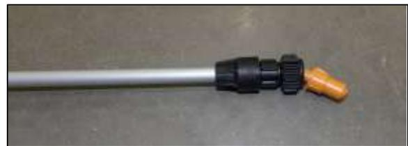
**Do not blow into the nozzle or poke wires into the tip to clear clogged holes. Replace the nozzle tip if it is damaged.**
