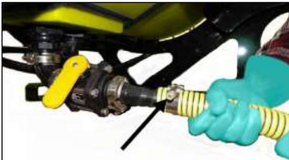
5. Slowly open the tank valve and allow the tank to completely drain.
