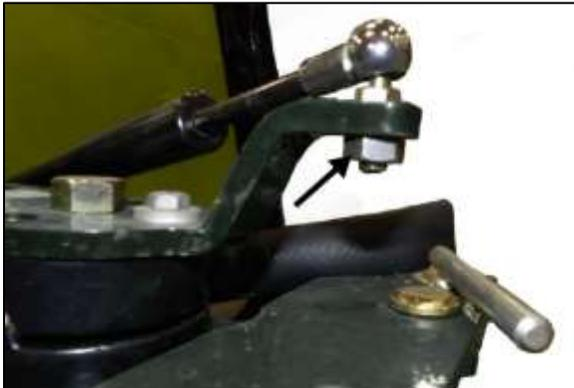
*Figure 18: Gas shock rod-end mounting*
