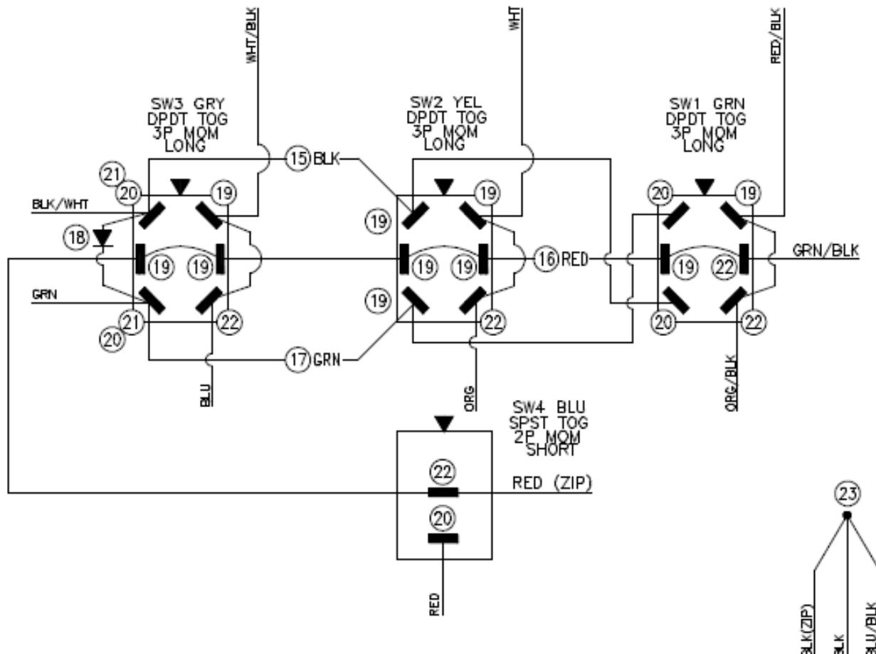
**Parts List: Cab Fold Box Electrical Wiring Diagram**
