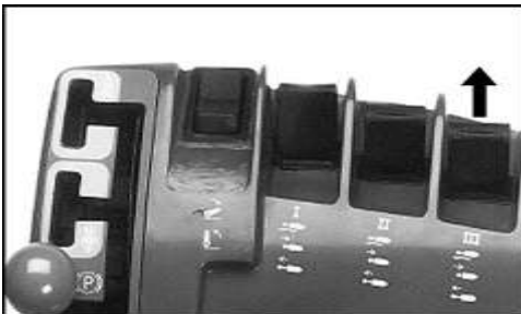
Figure 13: SCV III Pushed Forward
