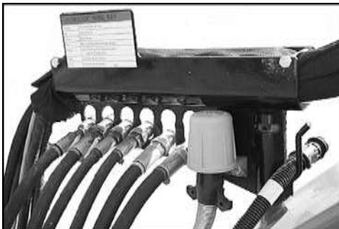
Figure 4: Wiring Harness and Hoses in Storage Position
