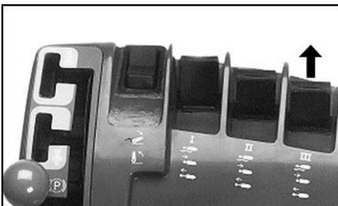
Figure 11: SCV III Pushed Forward
