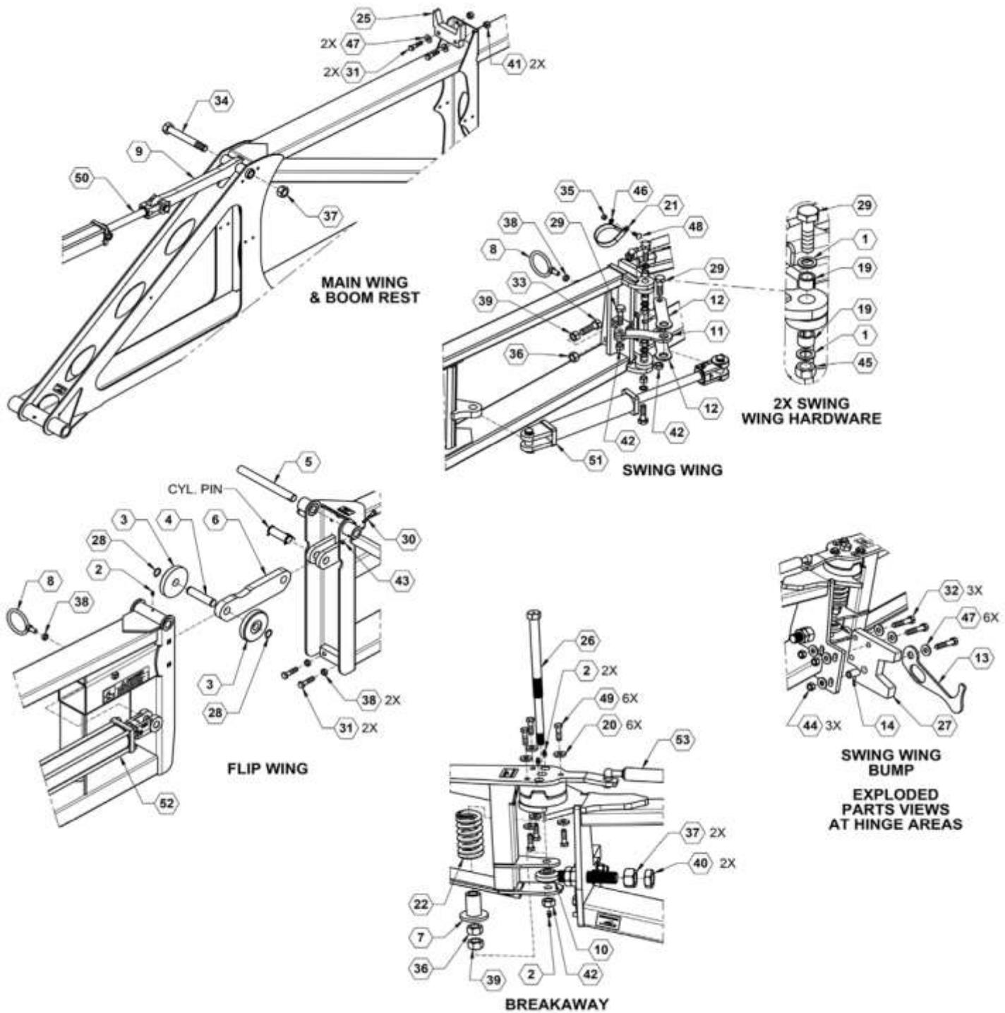
**Wings - Tri-Fold 40/80 Foot Boom Parts List**
