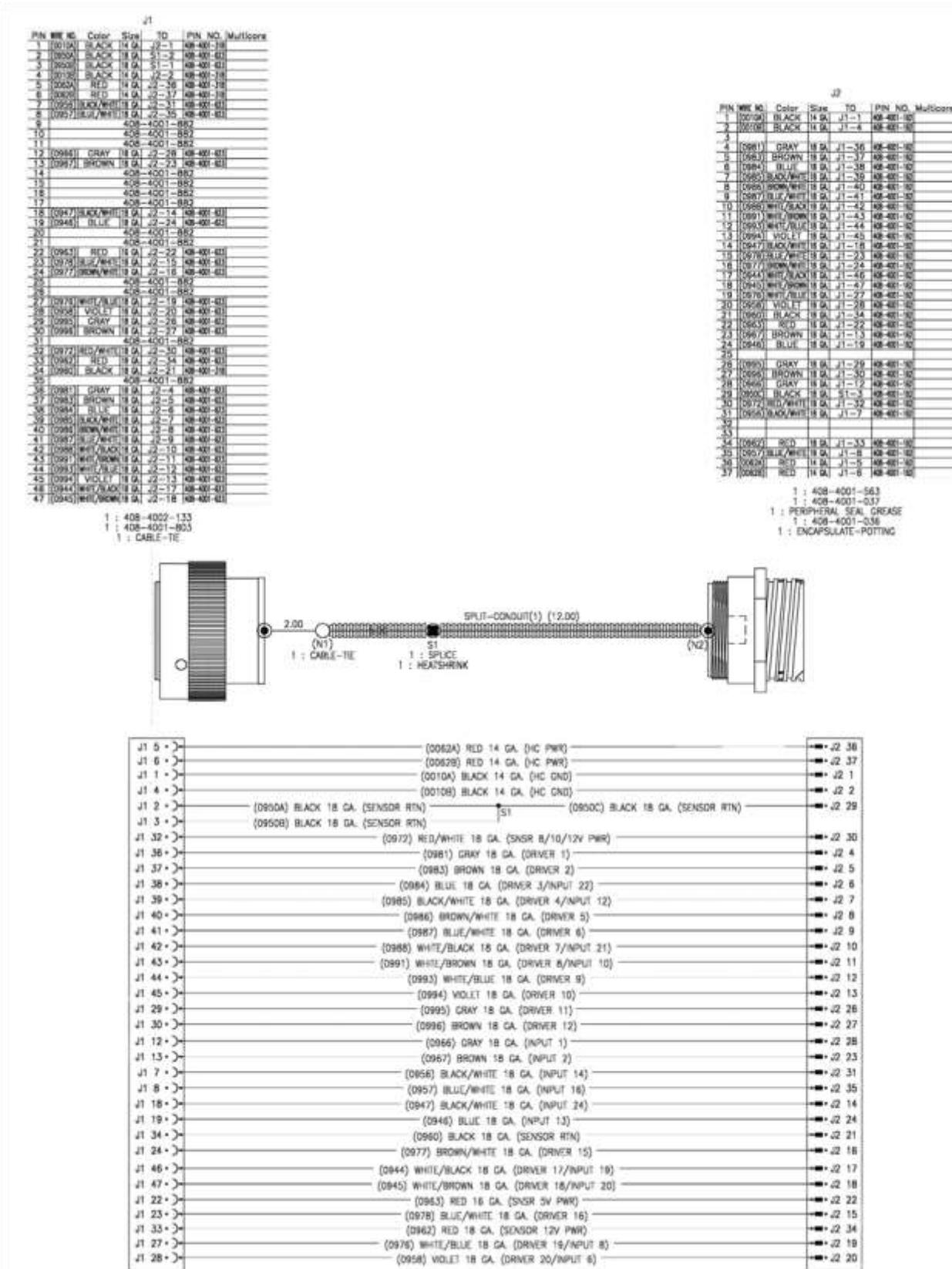
**Product Cable, 47 Pin, 6 Section, Liquid, FAST, Center Mount (632077)**
