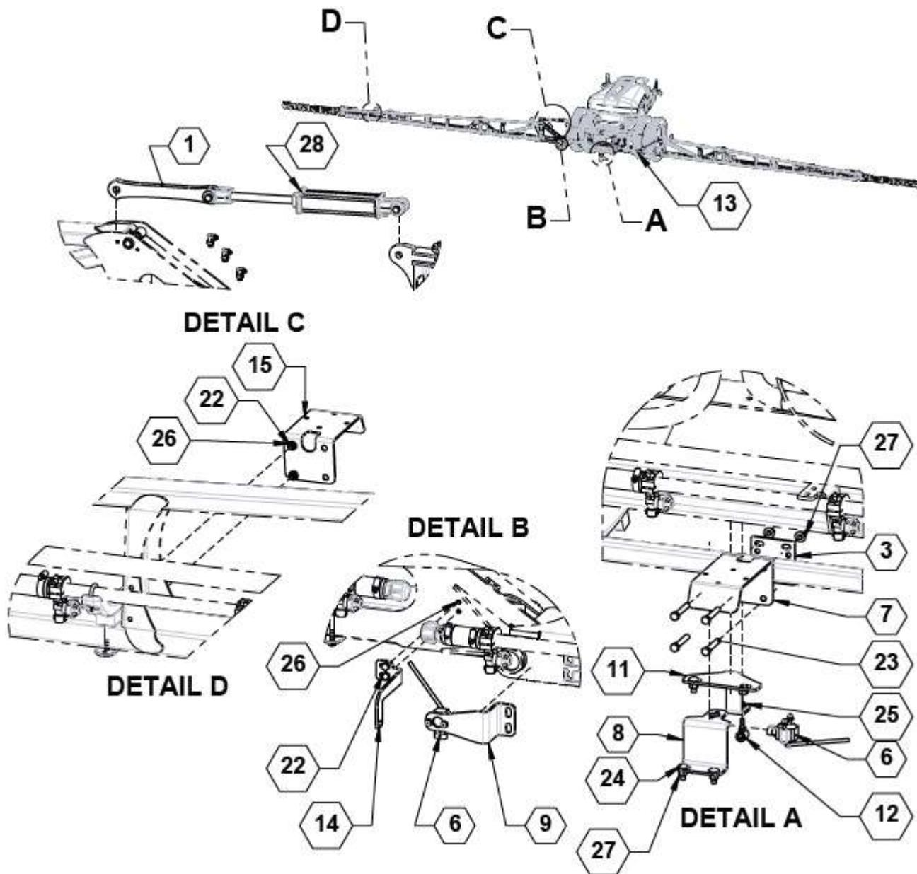
**Raven XRT Components, Tri-Fold Parts List 35900**
