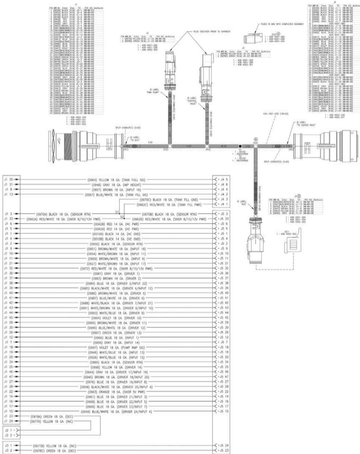
**Adapter Cable, 17', 9 Pin IBIC / 3 Pin Master to Gen 1 Isobus (632031)**
