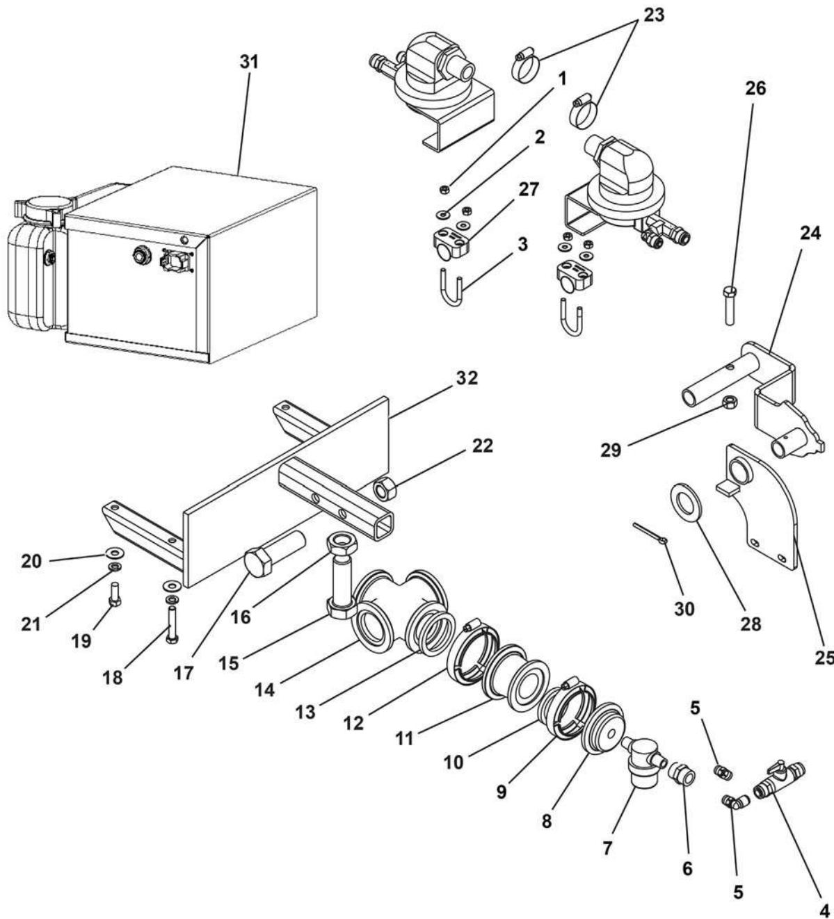
**Richway Direct Injection Foamer & Mounting Parts List**
