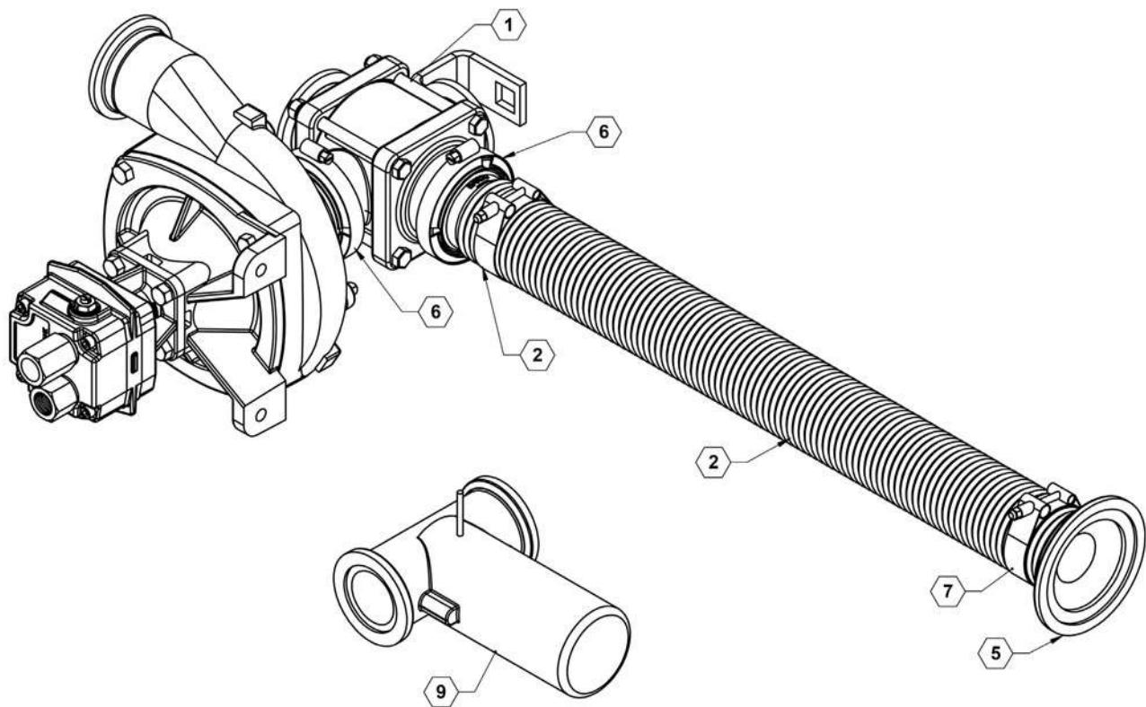
**Pump Option - 60' - 100' Boom With HYPRO Pump Pump Parts List**
