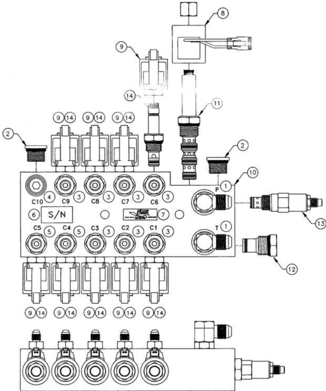
**Hydraulic Control Valve - 9600N Parts List**
