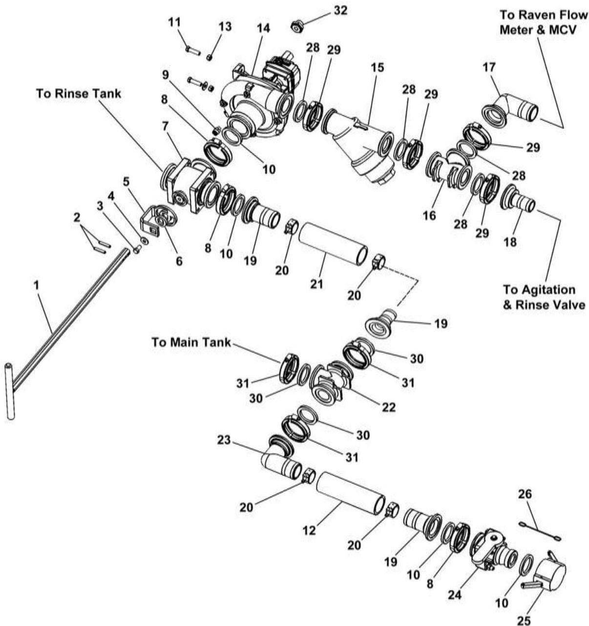
**Quick Fill & Pump Feed - 60-66 Ft Boom With ACE 150-206 Pump Parts List**
