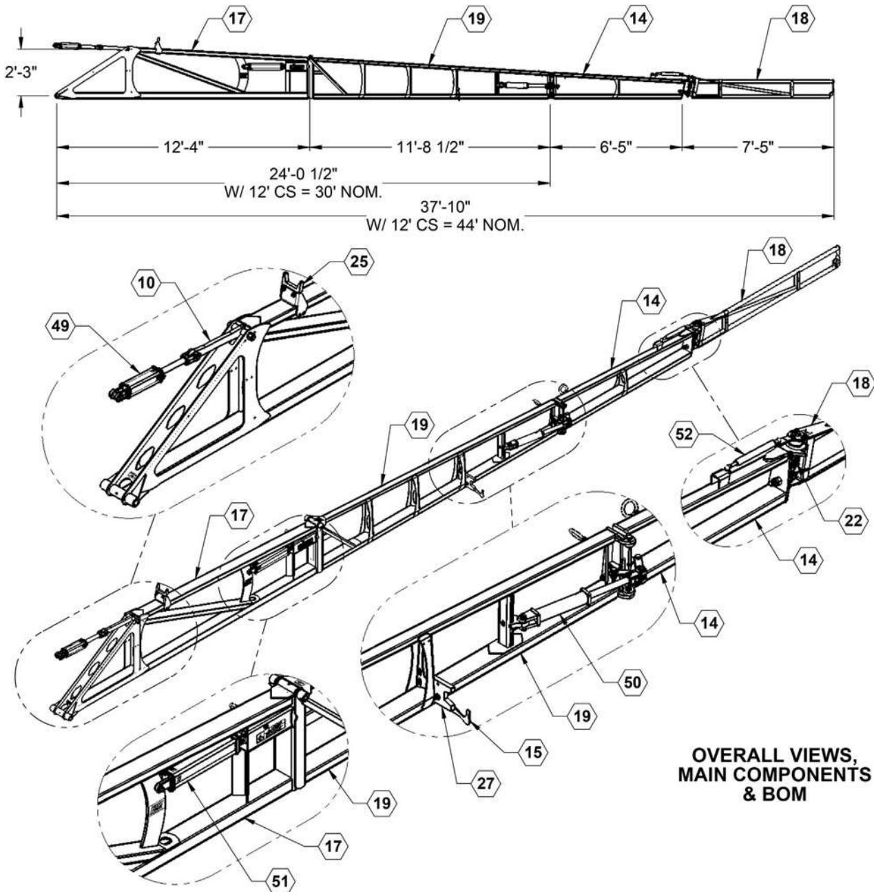
**Wings - Tri-Fold 60/88 Boom Parts List**
