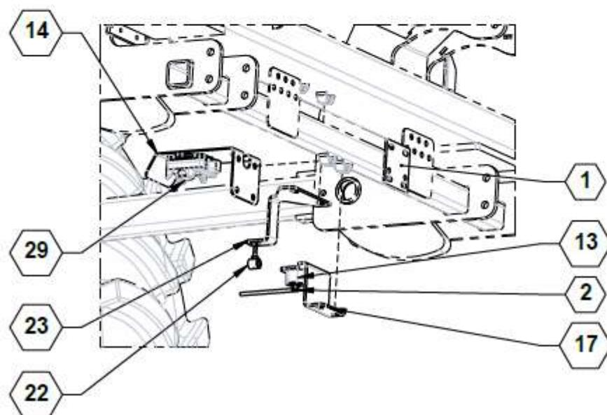
**Raven XRT Components, Truss Parts List 35901**
