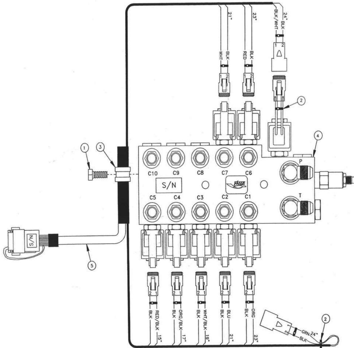
**Hydraulic Control Valve Harness - 60 - 66 Foot Boom Parts List**
