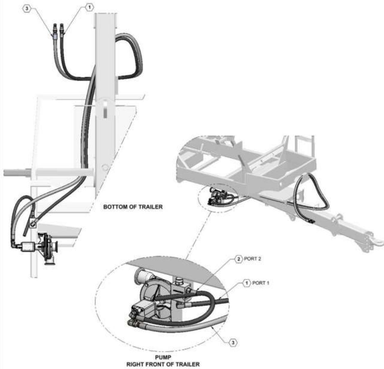
**Hydraulic Pump Hose Routing Parts List**
