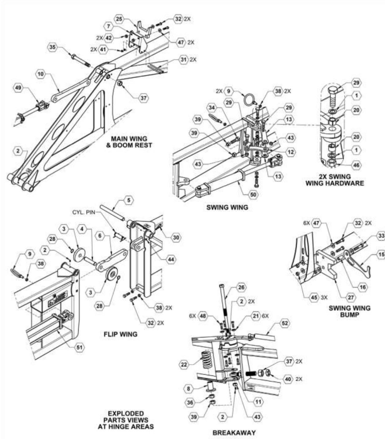
**Wings - Narrow Tri-Fold 60/90 Boom Parts List**
