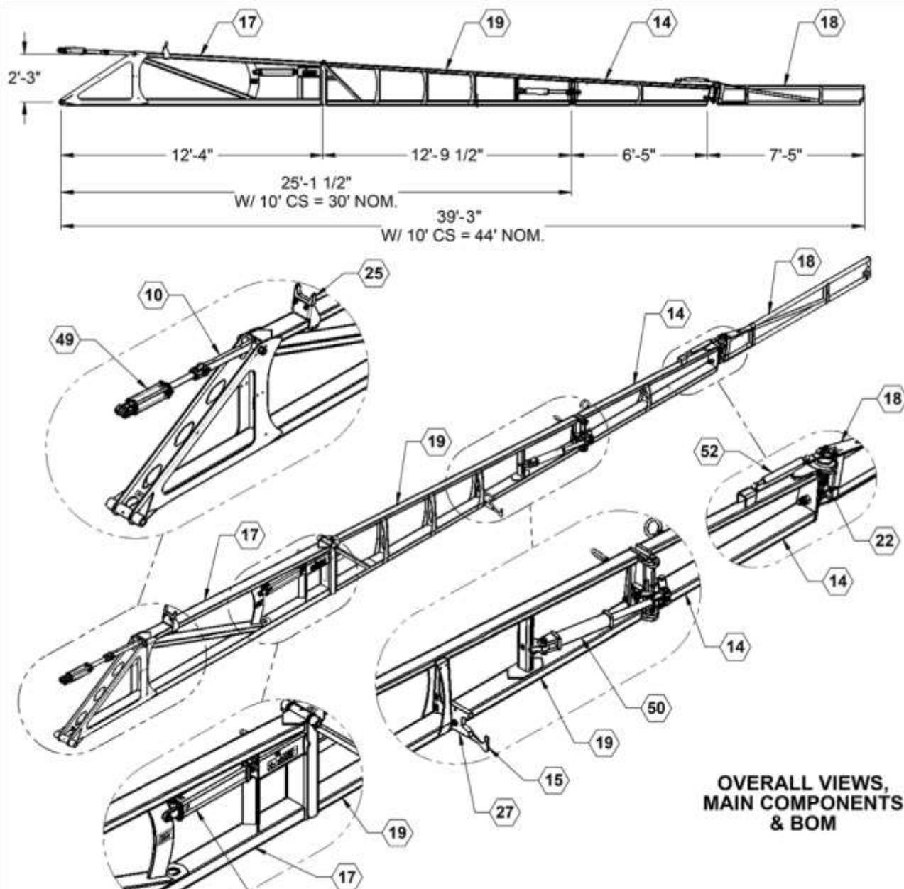
**Wings - Narrow Tri-Fold 60/88 Boom Parts List**
