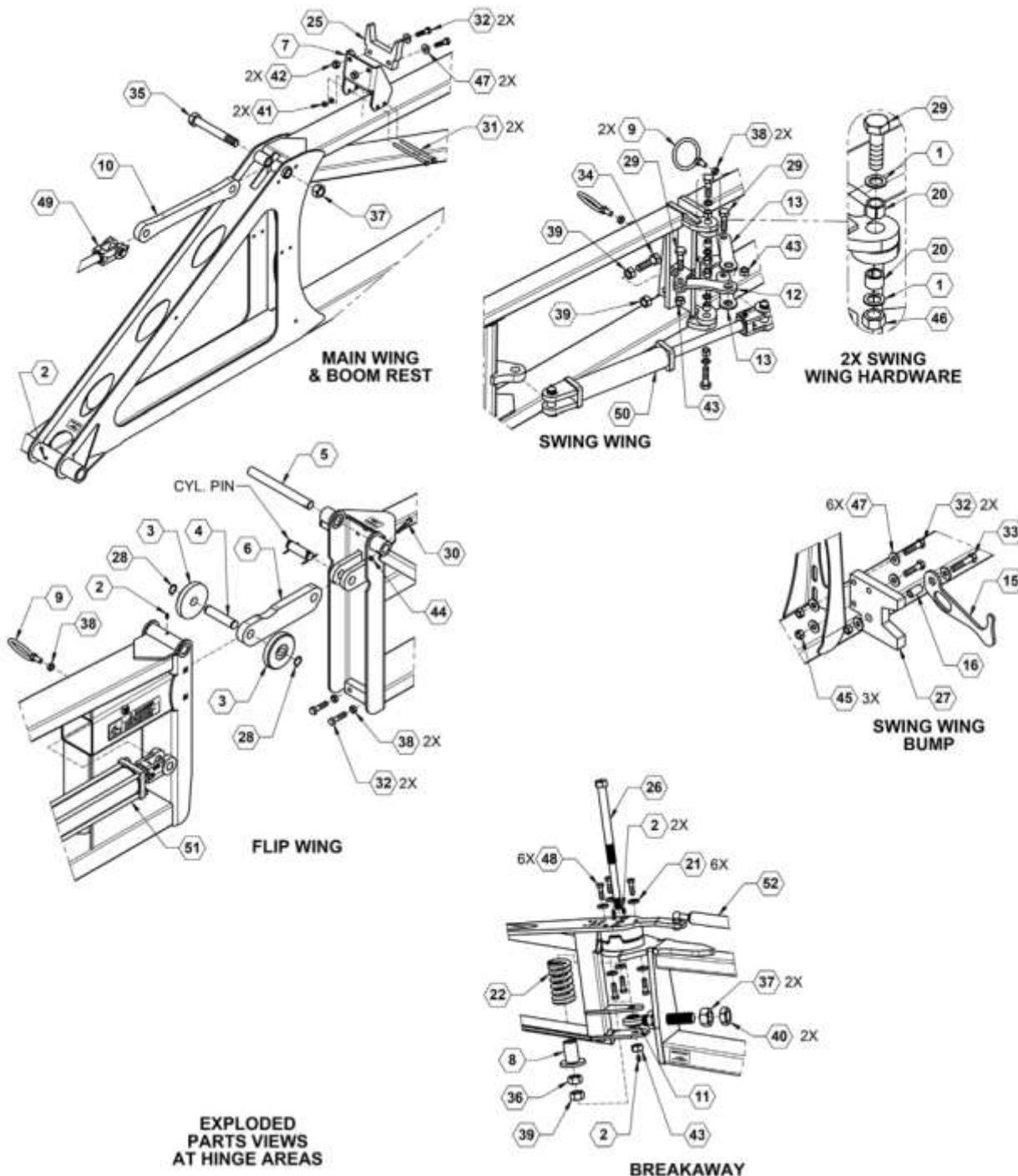
**Wings - Narrow Tri-Fold 60/88 Boom Parts List**
