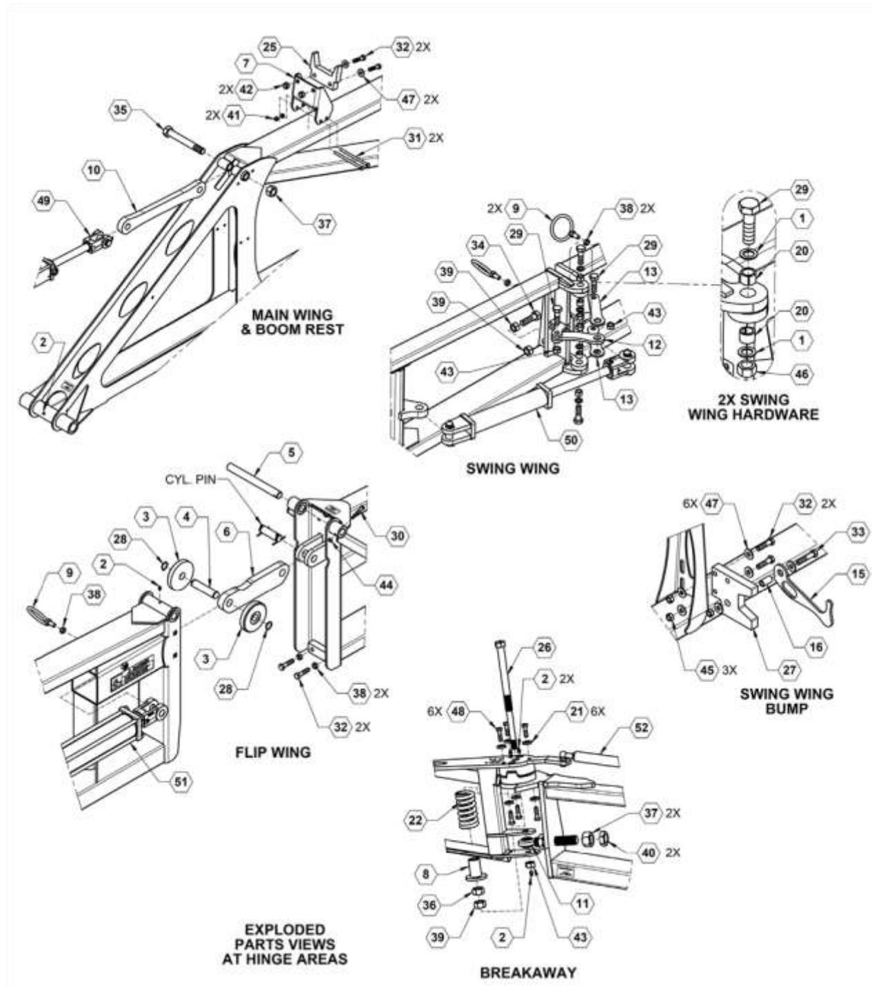
**Wings - Tri-Fold 60/90 Boom Parts List**
