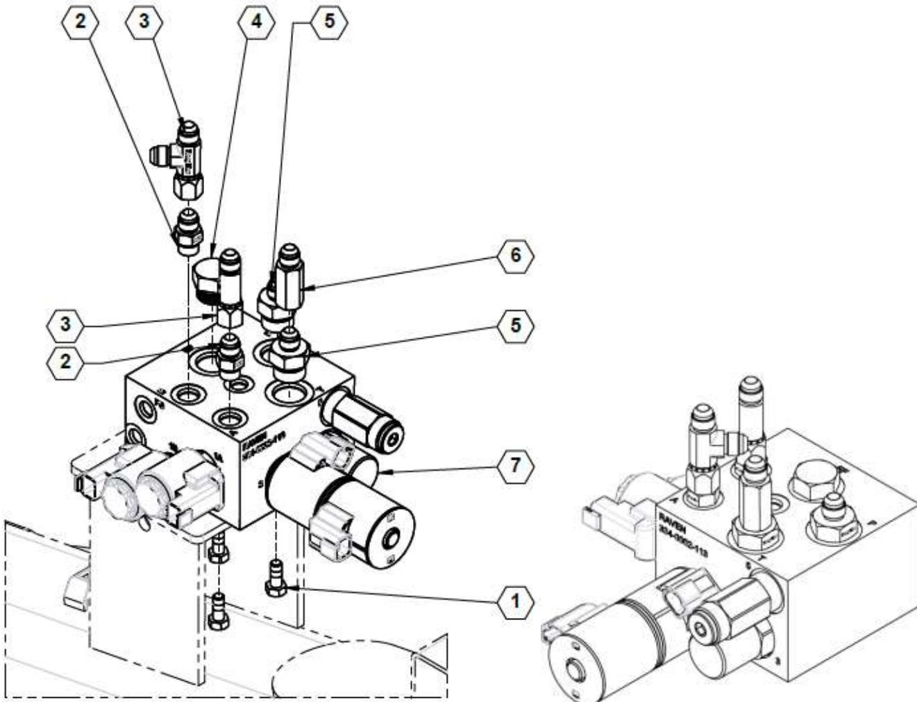
**Parts List 36685: Steerable Hitch Hydraulic Block**
