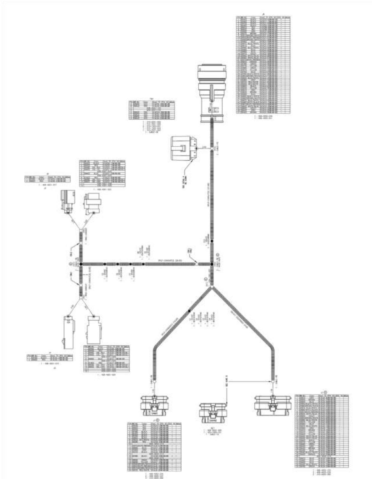
**Cable, 81 Pin ECU, 47 Pin Rate Control Interface (632029)**
