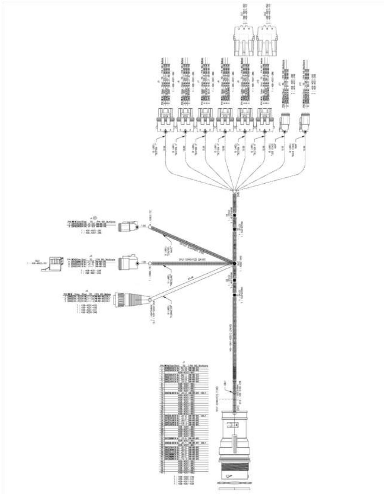
**Product Cable, 47 Pin, 6 Section, Liquid, FAST, Center Mount (632077)**
