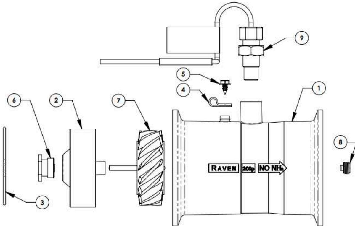
**Parts List 632125: High Flow Flowmeter Breakdown**
