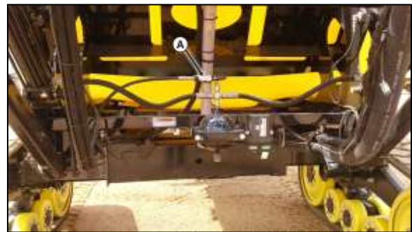
Figure 9: Boom lift shutoff valve above accumulator
