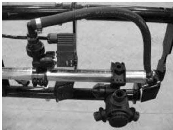
Figure 3: Electric shutoff fence row nozzle
