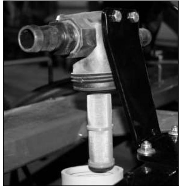
Figure 20: Typical boom line filter/strainer
