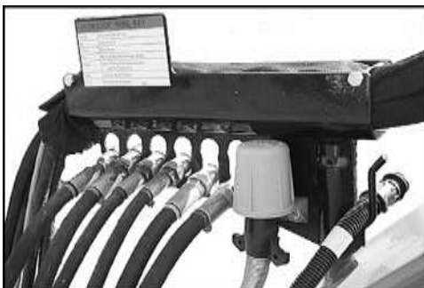
Figure 8: Wiring Harness and Hoses in Storage Position
