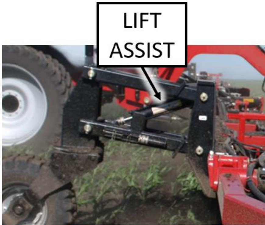
Figure 14: Toolbar Lift Assist cylinder in Right Lift Assist assembly
