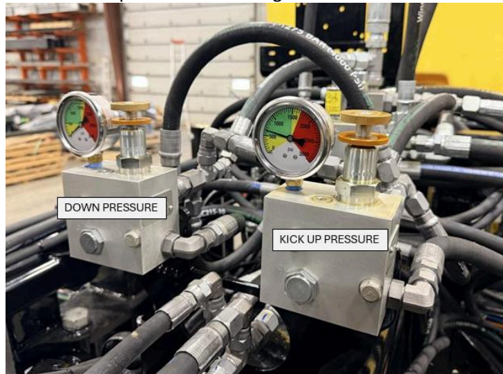
WING HYDRAULIC DOWN-PRESSURE AND KICK UP PRESSURE ADJUSTMENT AND GAUGES ON TOP OF TONGUE
