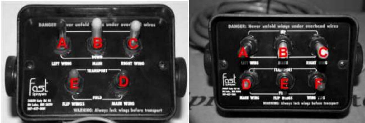
Figure 2: 5-function and 6-function control boxes
