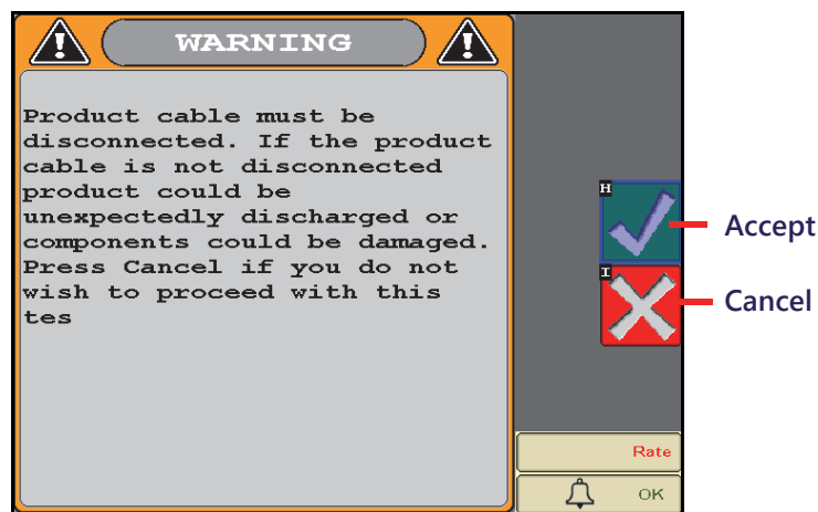
FIGURE 19. Loop Back Test Warning Prompt
