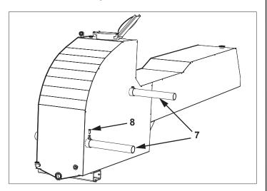
13. Reinstall step assembly and tighten all bolts on step tubes and tank.
