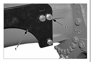
2. Install right rear tank support (3) to axle housing with three M16 x 40mm bolts (2) and M16 lock washers. Refer to torque charts in this instruction for bolt torque values.
