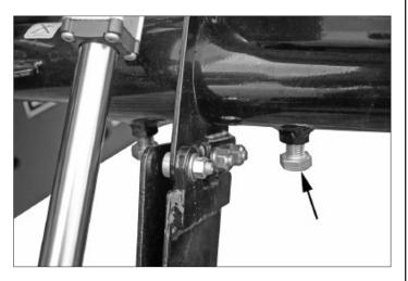
14. Insert ladder harness (9) in lower 3 inch tube and connect to existing tractor harness at side of motor and step.
