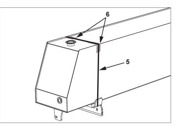
11. Tighten bolts on adjustable tank support cradles (item 6 on page 6).
