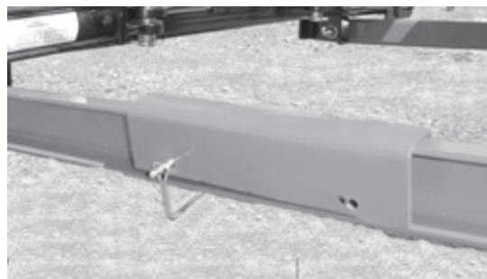
Transport Lock In Storage Position On Boom Stabilizer Arm
